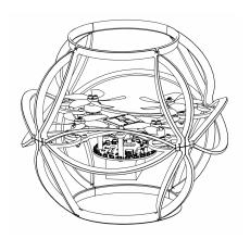
Maximum Total Weight: **300g**Frame Diameter **20cm** ± **2 (7.9in)**Maximum Base Truncation: **2cm**
